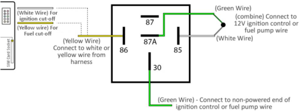
**NOTE: For ignition cut-off:** A constantly powered ignition control wire will need to be spliced (cut).
